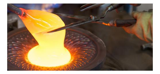
Images (left and right): 1. The flacon is sandblasted before being polished and satin-finished. 2. The right amount of molten crystal must be taken.
