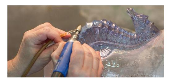
Images (left and right): 1. Rhinoceros, Nature Sauvage Collection. 2. The design and dimensions of the piece are defined by hand using a diamond-tipped tool.
